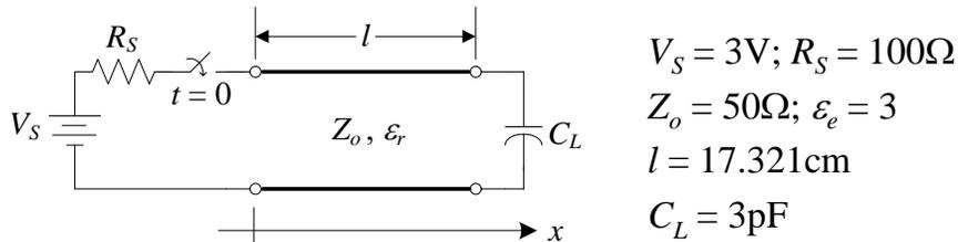
$$V_o^+ = V_S Z_o / (R_S + Z_o) = 1\text{V}$$
