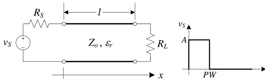
$$R_S = 75\Omega; R_L = 30\Omega; A = 3V; PW = 2.5\text{ns}$$
