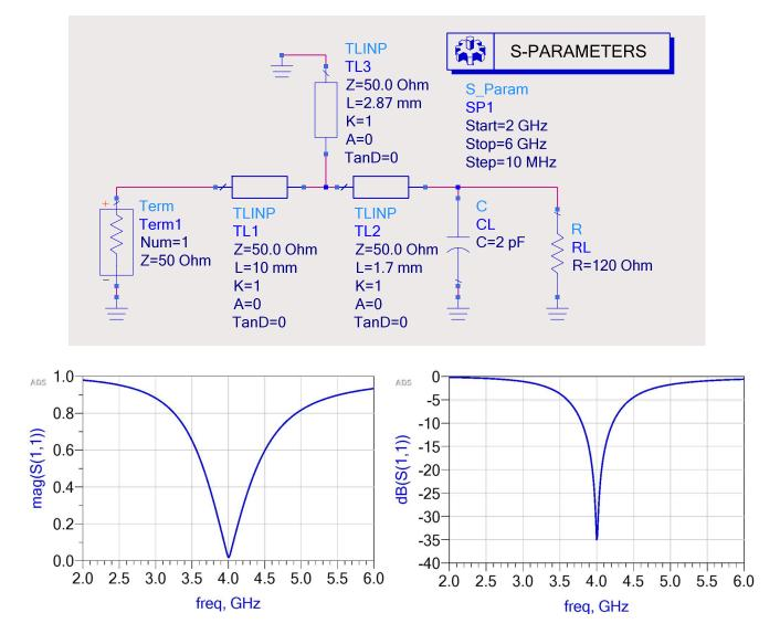
It is seen that Solution 2 provides a larger matching bandwidth than Solution 1.
