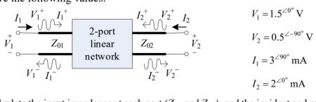
Calculate the input impedance at each port ( $Z_{in1}$  and  $Z_{in2}$ ), and the incident and reflected voltage waves at each port ( $V_1^+$ ,  $V_1^-$ ,  $V_2^+$ , and  $V_2^-$ ), measured with respect to a reference impedance of  $Z_{01} = Z_{02} = 50 \Omega$ .
