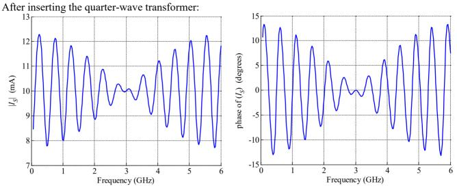
Notice that, after inserting the quarter-wave transformer, the magnitude of  $I_S$  becomes less sensitive to the frequency around 3 GHz ( $|I_S| = |V_S|/(R_S + Z_1) = 10$  mA at 3 GHz), and the phase of  $I_S$  is almost 0° around 3 GHz (because  $Z_{in}$  is resistive around 3 GHz, since  $Z_{in} = Z_1 = 50 \Omega$  at 3 GHz).
