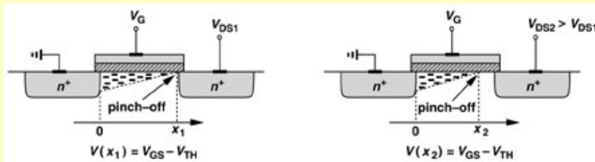
Minimum channel density occurs when  $v_{GS} - V(x) = V_{TH}$
