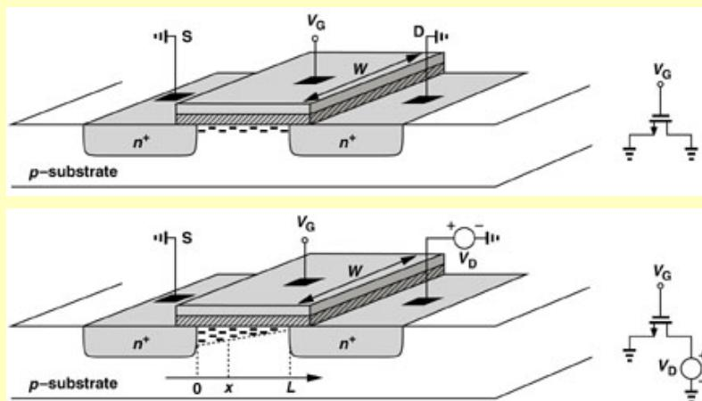
Channel thickness depends on  $v_{GS} - V(x)$
