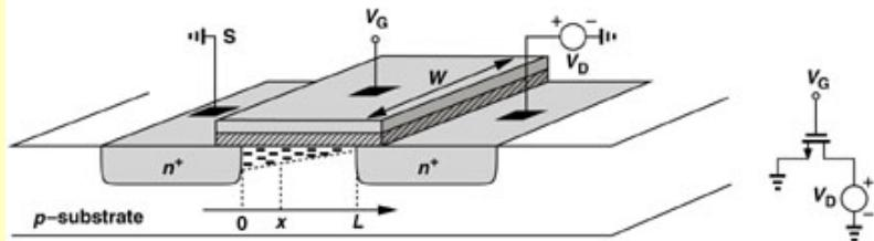
Channel density at  $x$  depends on  $v_{GS} - V(x)$
