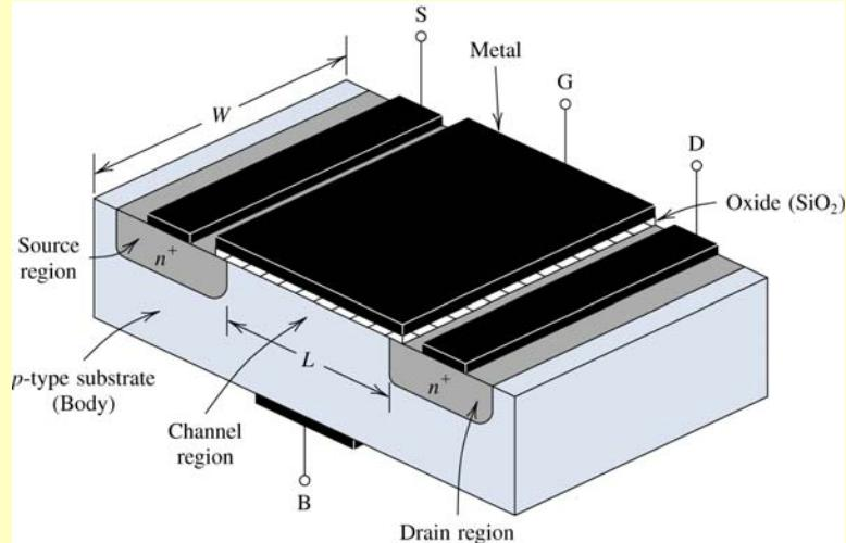
Typical dimensions:  $0.1\mu\text{m} \leq L \leq 10\mu\text{m}$
