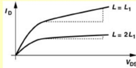
Larger MOSFETs are less sensitive to the channel length modulation effect
