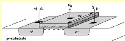
$$Q_d = -WC_{OX}(v_{GS} - V_{TH})$$
