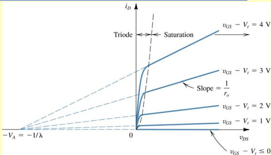
$$i_{DS} = \frac{1}{2} \mu_n C_{ox} \frac{W}{L} (v_{GS} - V_{TH})^2 (1 + \lambda v_{DS})$$
