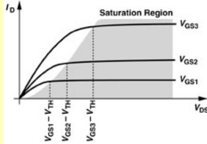
$$i_{DS} = \frac{1}{2} \mu_n C_{ox} \frac{W}{L} (v_{GS} - V_{TH})^2$$
