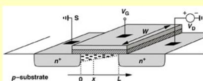
$$Q_d = -WC_{OX}[v_{GS} - V(x) - V_{TH}]$$
