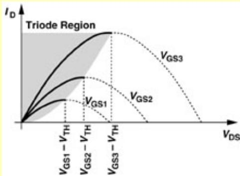
The peak of each parabola occurs at  $v_{DS} = v_{GS} - V_{TH}$
