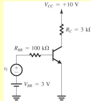
$$\begin{aligned}\beta &= 100 \\ \eta &= 1 \\ g_m &= 92 \text{ mΩ}^{-1} \\ r_\pi &= 1.087 \text{ kΩ}\end{aligned}$$
