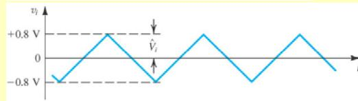
$$i_b = \frac{v_i}{R_{BB} + r_\pi} = \frac{0.8 \text{ V}}{100 \text{ kΩ} + 1.087 \text{ kΩ}} = 7.914 \text{ μA}$$
