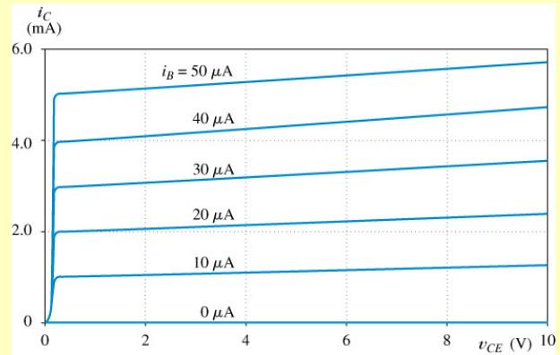
$i_C$  increases with  $v_{CE}$  due to the Early effect
