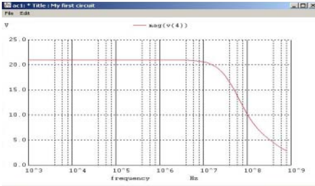
Fig 10. AC simulation of the CMOS feedback amplifier (with \lambda = 0 ) increasing the values of W and L by a factor of 10.
