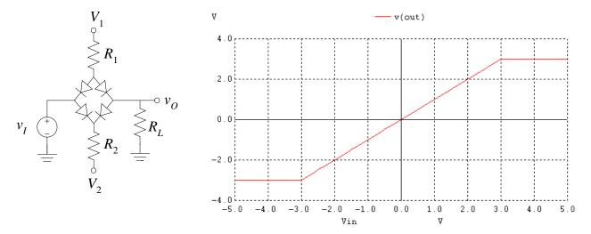
Apply a 5V, 1KHz, sinusoidal input signal and plot the output voltage from 0 to 4 ms, using a plotting time step of 1µs:
