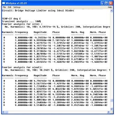
Now use diodes 1N4004 and repeat the analysis. Notice that the Total Harmonic Distortion at the output increased from THD=18.54% to THD=21.60%
