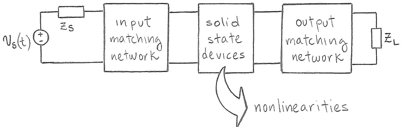
$v_s(t)$  is typically a sinusoidal source with a DC bias component, but could be any waveform
