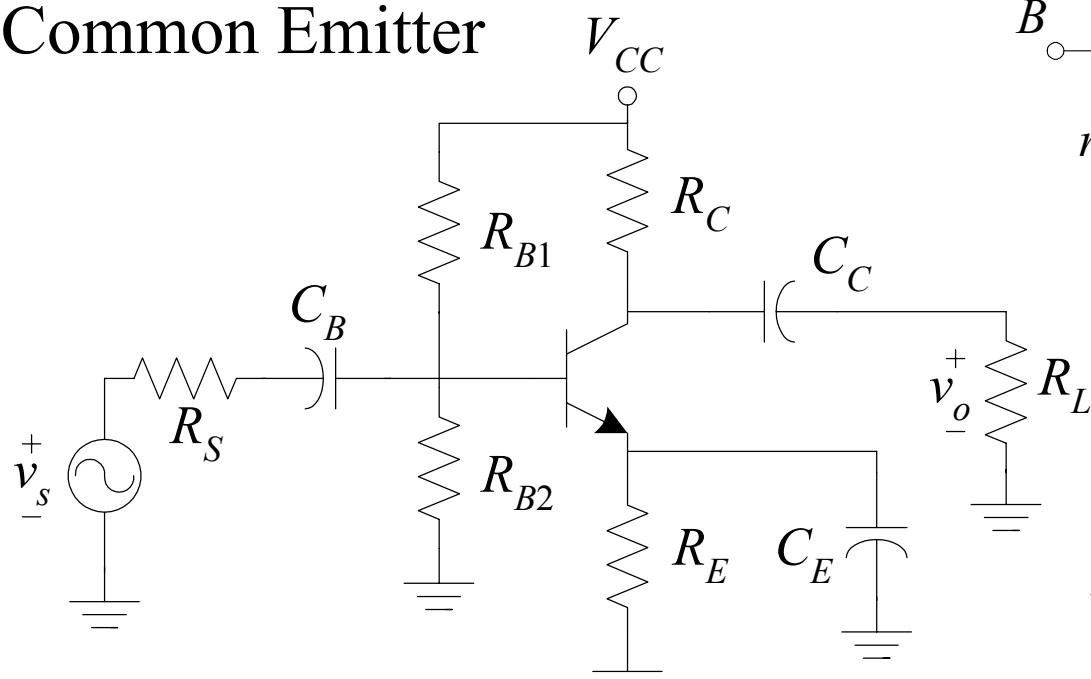
$$\omega_L \approx \frac{1}{R_{C_B} C_B} + \frac{1}{R_{C_E} C_E} + \frac{1}{R_{C_C} C_C}$$
