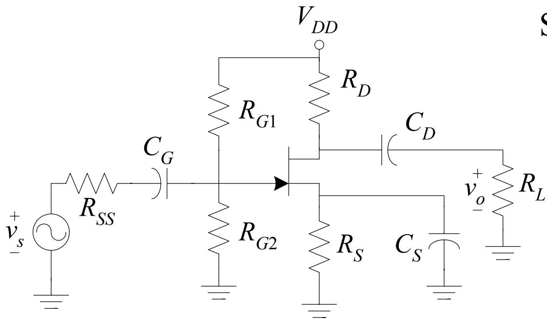
$$\omega_{P1} = \frac{1}{[R_{SS} + (R_{G1} \parallel R_{G2})]C_G}$$
