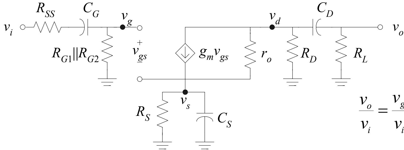
$$v_s = i_s Z_s = [g_m v_{gs} + (v_d - v_s)/r_o] Z_s = [g_m v_g + v_d/r_o - v_s(g_m + 1/r_o)] Z_s$$
