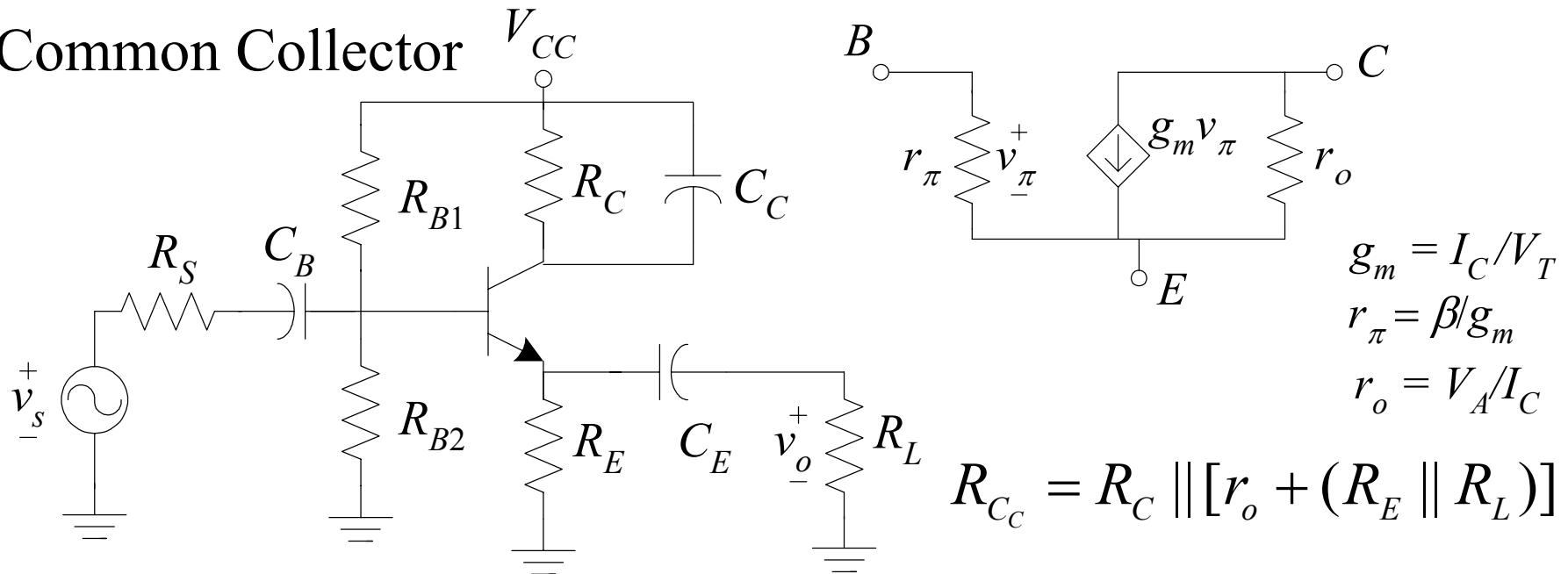
$$\omega_L \approx \frac{1}{R_{C_B} C_B} + \frac{1}{R_{C_E} C_E} + \frac{1}{R_{C_C} C_C}$$
