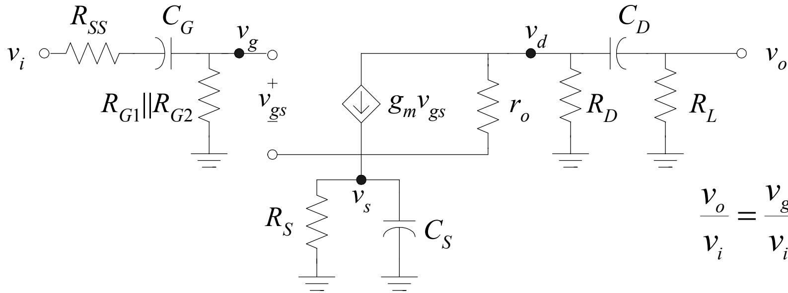
$$v_g = \frac{(R_{G1} \| R_{G2})v_i}{R_{SS} + (R_{G1} \| R_{G2}) + 1/sC_G}$$
