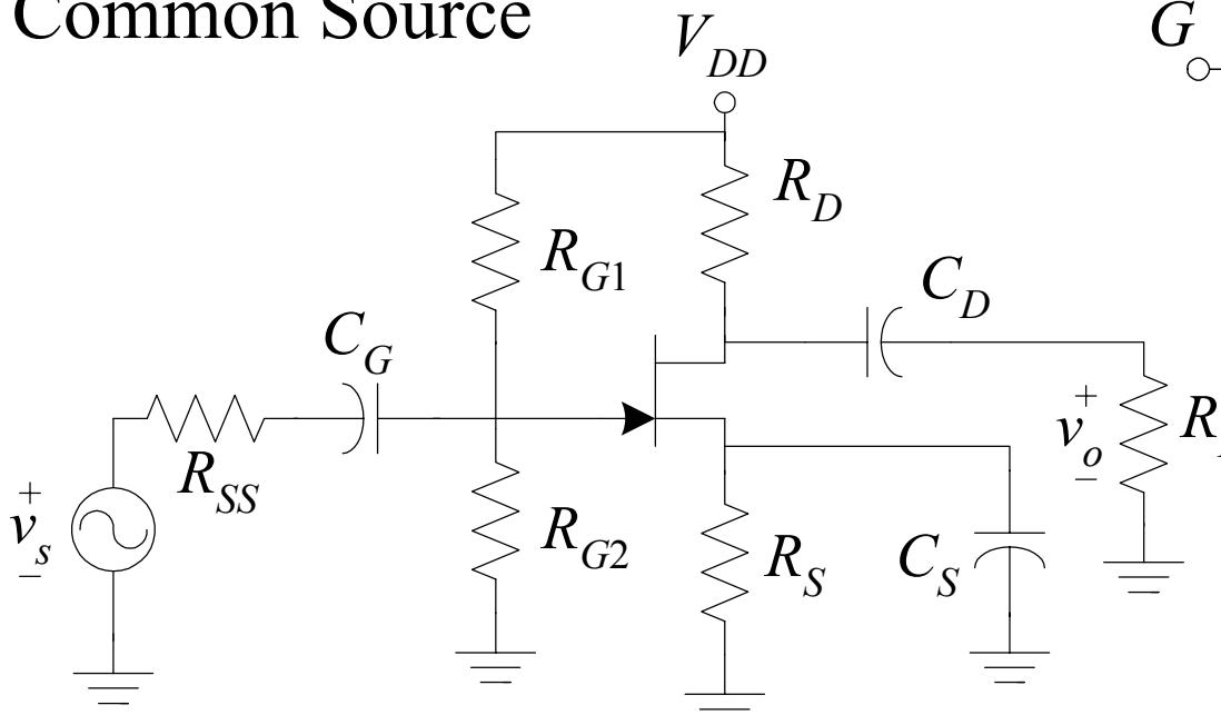
$$\omega_L \approx \frac{1}{R_{C_G} C_G} + \frac{1}{R_{C_S} C_S} + \frac{1}{R_{C_D} C_D}$$
