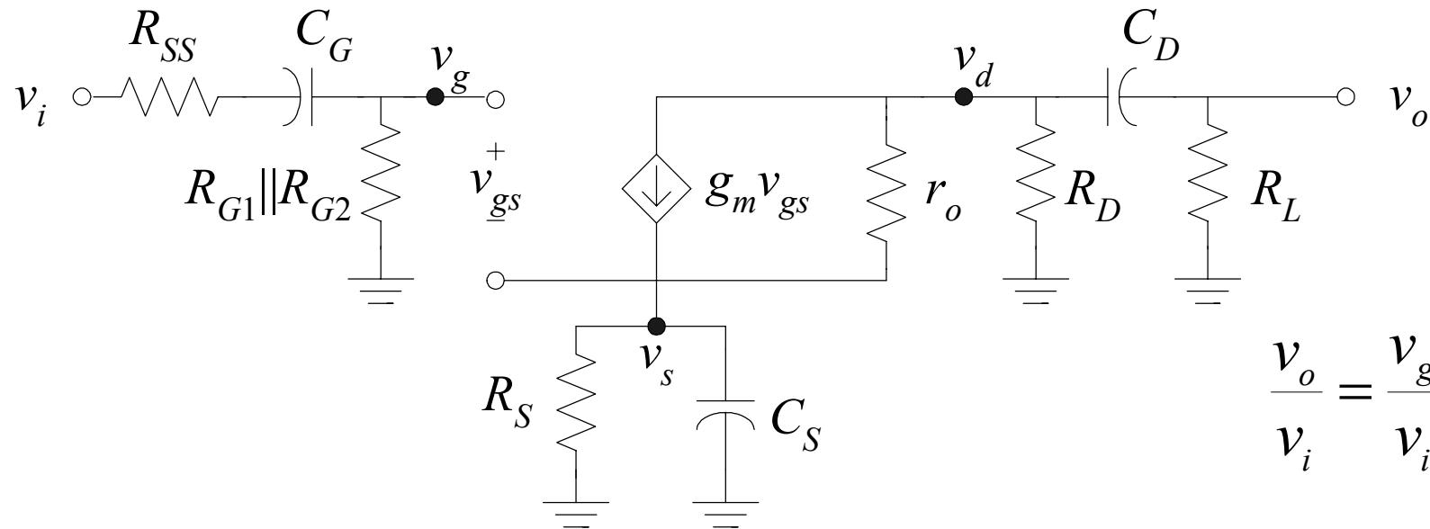
$$\frac{v_o}{v_i} = \frac{v_g}{v_i} \frac{v_s}{v_g} \frac{v_d}{v_s} \frac{v_o}{v_d}$$
